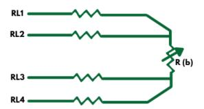
Ohm's law can be used to determine the exact measuring resistance by dividing the measuring voltage by the constant current. Umeas / I = Rmeas
