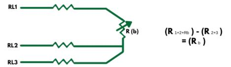
The resistance is calculated by first calculating the resistance between wires 1 and 2 and then subtracting the resistance between wires 2 and 3 which results in an accurate measurement for the resistance element (Rb). This method assumes that all wires are measuring the same resistance; they therefore must be identical.
